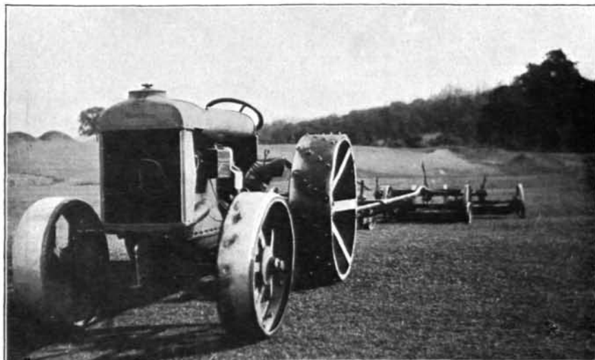
Tractor used at the Glen Echo Country Club. Note the altered front wheel and spiked rear wheel
