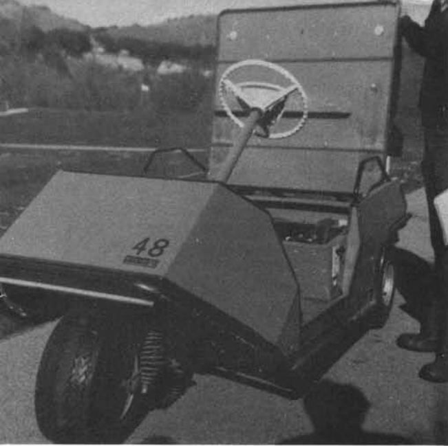
A three-wheel car with the seat showing the batteries position.
