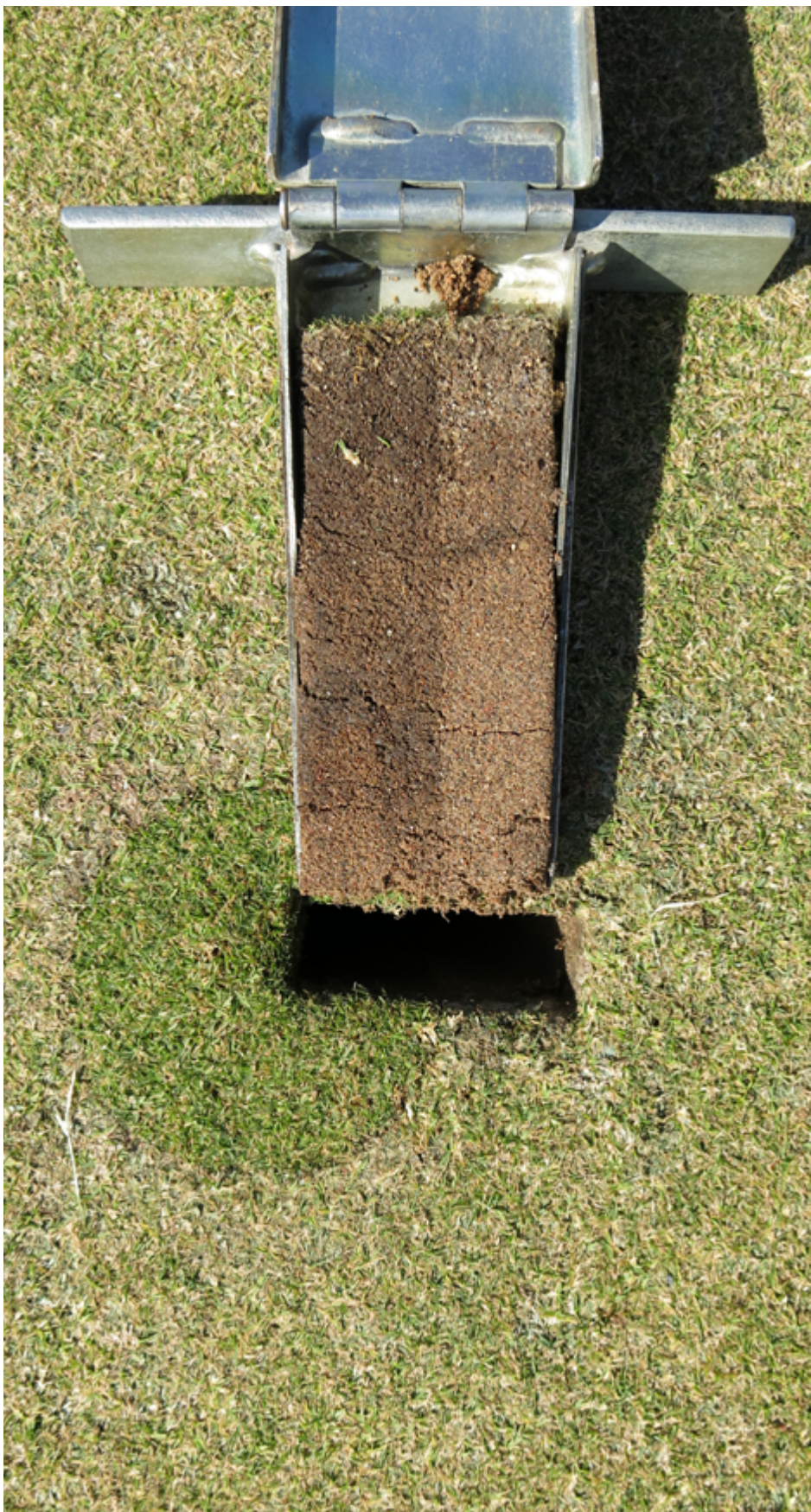
The plug in this image was moved from the original portion of this green into an expansion area. The rootzone mixtures do not match in performance characteristics, so turf quality does not match either.
