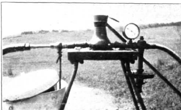
Applying carbon disulfid emulsion prepared in a proportioning machine. The machine is shown on the reader's right.
