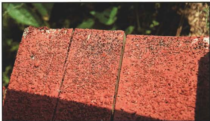
A combination of fast-drying epoxy paint and sand-blasting material can be used to create and preserve a textured surface. When the combination dries, the surface is wear tolerant, aesthetically acceptable, and coarse textured.
