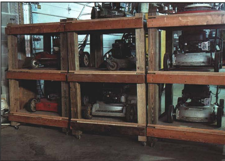
Mounting swivel casters under multi-shelf storage racks will optimize the workspace in any size maintenance facility.
