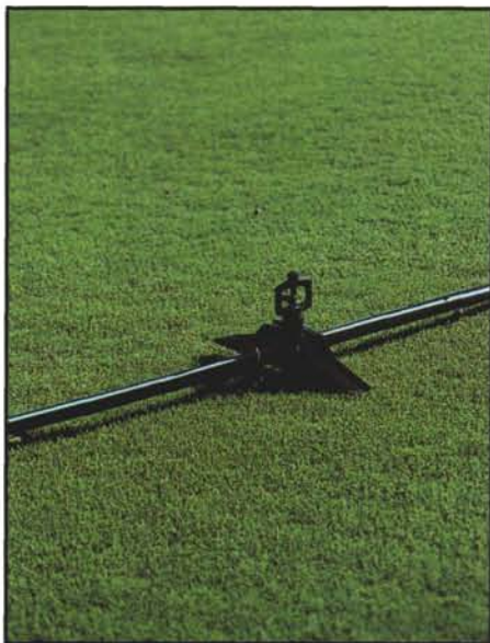
Low-volume sprinklers can be used to leach native soil greens without causing runoff into bunkers and green surrounds. These sprinklers are available from several manufacturers, with application rates ranging from 0.5 to 1.0 gallon per minute and a radius of 12 to 15 feet. See page 26.
