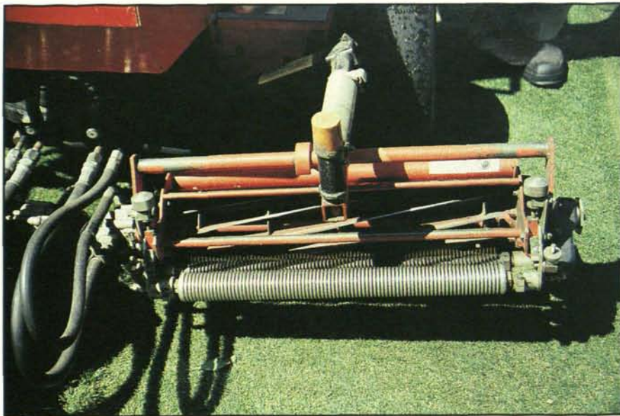
Above: Grooming attachments can be beneficial in encouraging a more upright growth habit, but they add weight directly to the cutting unit and can increase wear injury. Below: Some superintendents have reduced five-plex ring problems by altering the cutting units. In this instance, the original front (Wiehle) and rear rollers have been replaced with lighter solid rollers from a putting green mower. A weight bar has also been removed.
