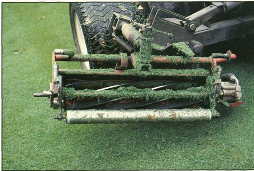
Above: Grooming attachments can be beneficial in encouraging a more upright growth habit, but they add weight directly to the cutting unit and can increase wear injury. Below: Some superintendents have reduced five-plex ring problems by altering the cutting units. In this instance, the original front (Wiehle) and rear rollers have been replaced with lighter solid rollers from a putting green mower. A weight bar has also been removed.
