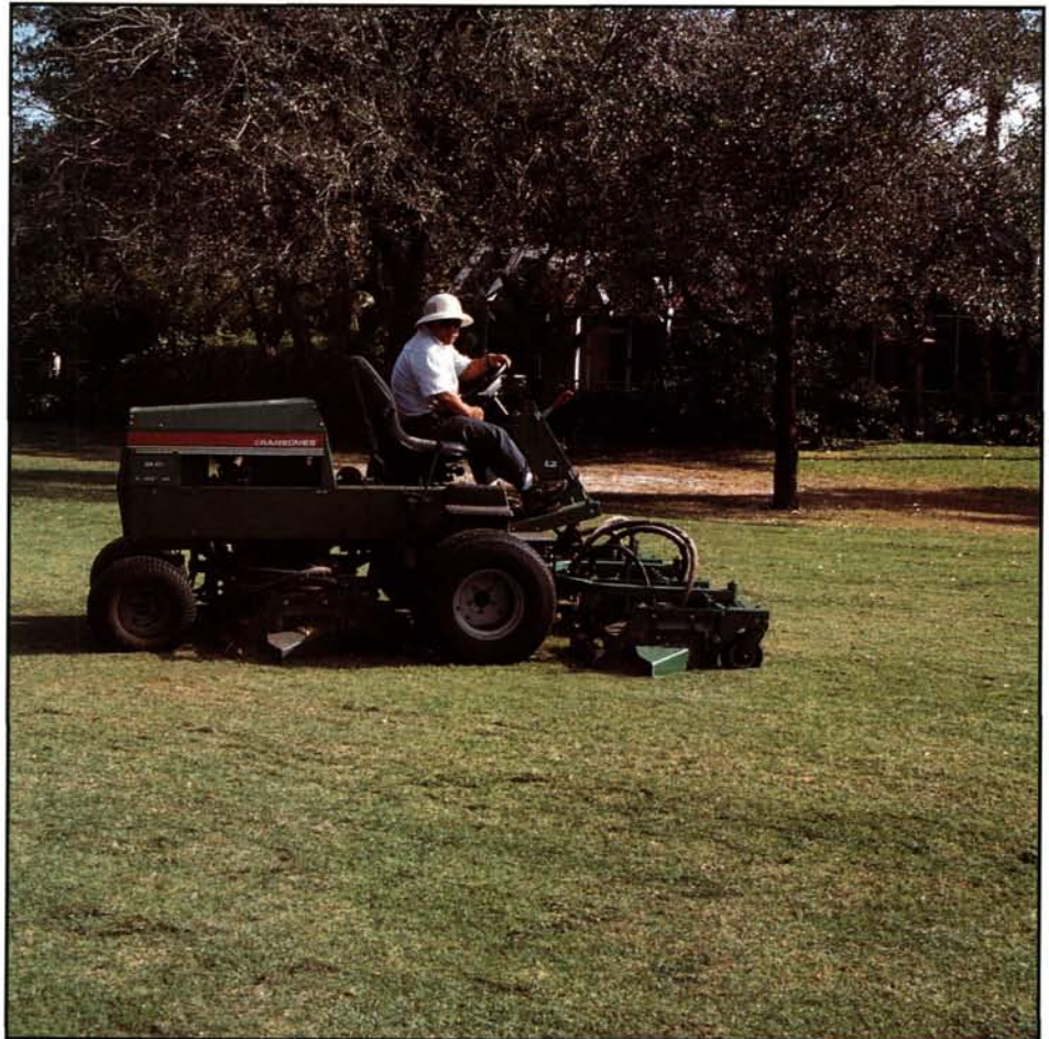
Over the past few years, the use of rotary mowers to maintain hybrid bermudagrass roughs has been a growing trend. To maintain a good quality cut, the blades must be sharpened on a regular basis.
