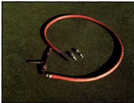
Left: The hose system consists of a 6-foot length of \frac{3}{4} - or 1-inch hose attached to a quick coupler. The nozzle can be made with reducing couplers and nylon reducing inserts as shown or with a \frac{3}{4} -inch aerification tine clamped directly to the hose. Right: A \frac{3}{4} -inch hollow tine clamped directly to the hose works well as a nozzle.
