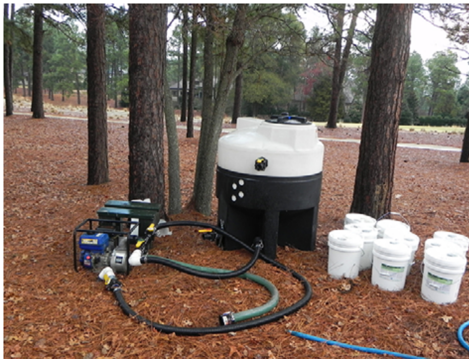
A pre-mixing tank mixes turf colorants with water and quickly fills the sprayer. Tanks can be moved to any location on the golf course to speed sprayer operations.
