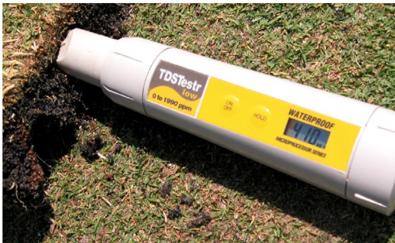
Portable salt meters are excellent tools for quickly and easily monitoring salt levels throughout the soil profile.
